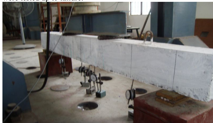
Fig 5 Experimental Setup for the Flexure Beam
