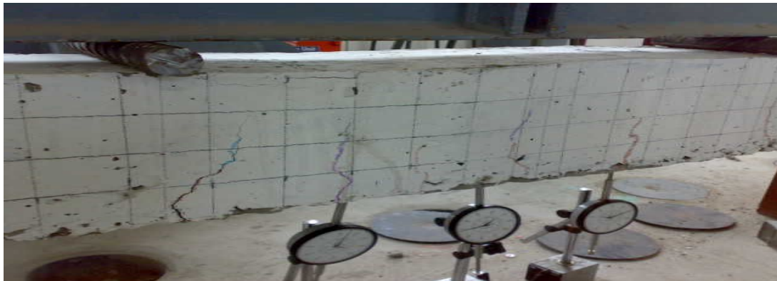
Fig 10 Crack pattern for the beam for flexure after loading
