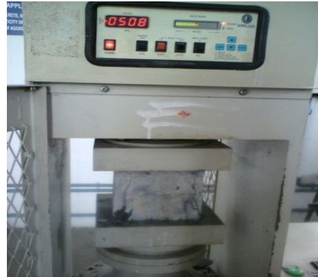
Fig.4 Testing of Cubes in CTM
